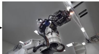
Automated Fiber Placement
